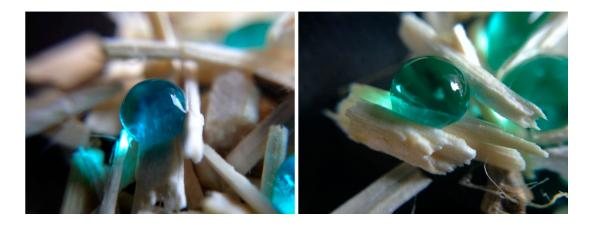
Figure 8. Coloured water droplets onto hemp shiv H12-1-5, with a WCA > 125°. Courtesy of TWI Ltd.
